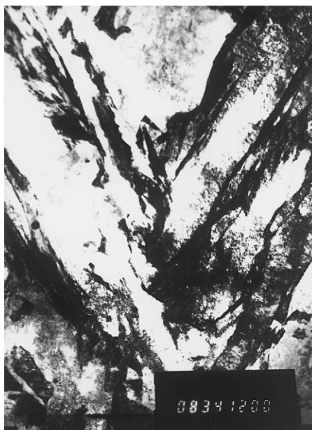
Fig. 1. Microstructure of 0.1C-9Cr-1W, V, Ta in the unirradiated condition.
