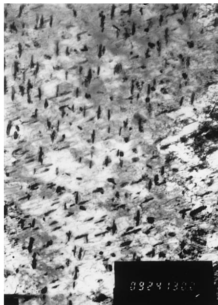
Fig. 2. Secondary phases precipitation in unirradiated steel.
